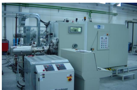
Figure 13 Assender's Roll-to-Roll Deposition Tool in Begbroke Science Park
